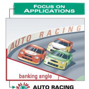
Banked turns help the cars travel around the track at high speeds. The angles provide an inward force that helps keep the cars from flying off the track.
